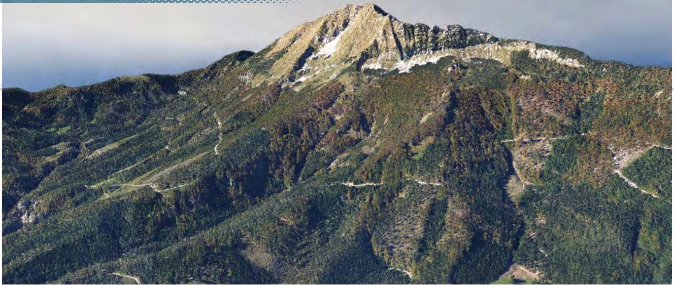
Colored Point Cloud, Ötztal, Austria, acquired in 2012 by an LMS-Q780. 57 km 2 scan area; 716 million points; 13 points/m 2 average point density; 27 minute scan time.
