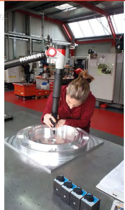
6-axis measuring tool being used to check the machining of a base plate for an LMS-Q1560.
