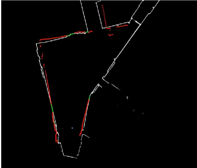
Illustration of the Localization process on the left, where the red instant measurement has to match the white map—Illustration of map result on the right.
