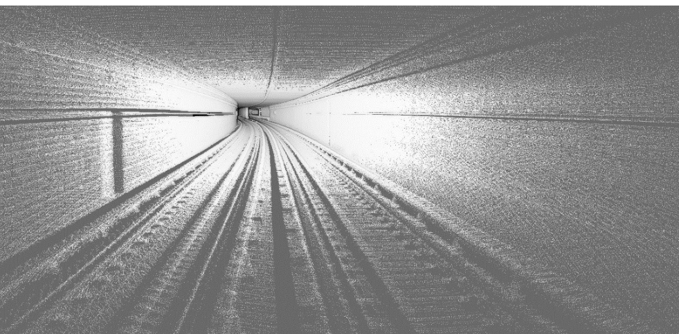
Tunnel scanning is difficult to handle with only SLAM approach—Features inside are too small to eliminate the ambiguity
