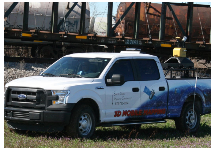
Sorrell-Smith's Charlie Patton and Jerrad Burns prepare the Topcon IP-S3 for a scanning session.
