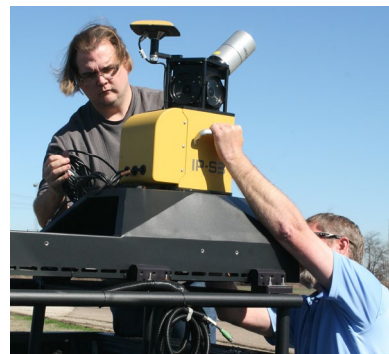
Sorrell-Smith's Charlie Patton and Jerrad Burns prepare the Topcon IP-S3 for a scanning session.
