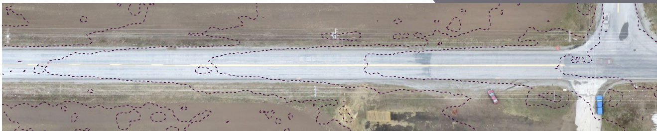
UAV photogrammetric survey of Huetter Road with contours.
