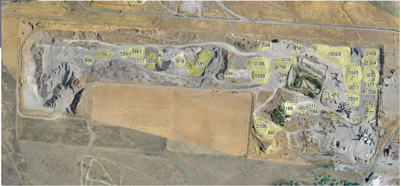
Open-pit quarry with gravel pile quantities.
