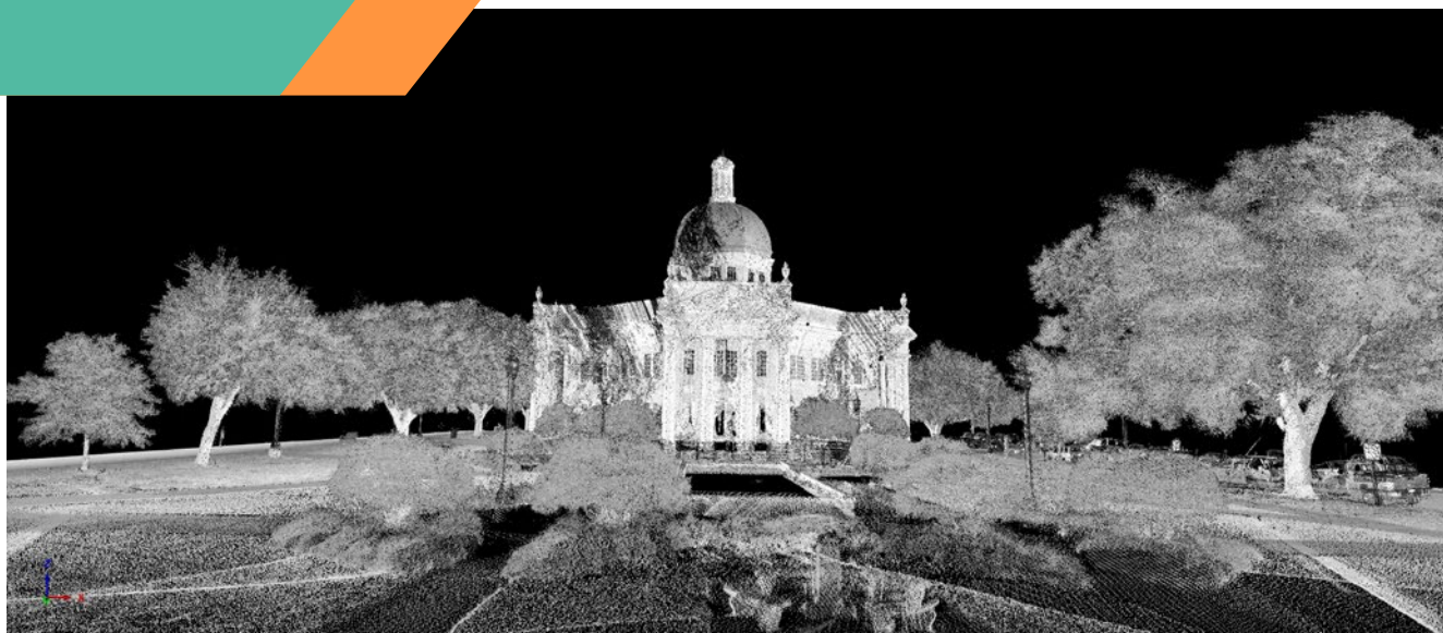
Above: LiDAR point cloud collected from the Riegl VMX-450 of the Aubrey K. Lucas Administration Building at USM.
