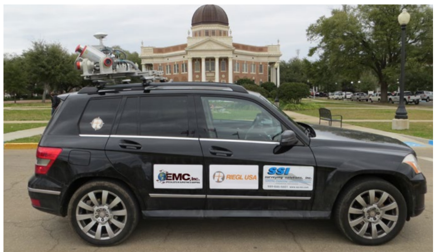
The Riegl VMX-450 mobile mapping system on the University of Southern Mississippi's Hattiesburg campus.
