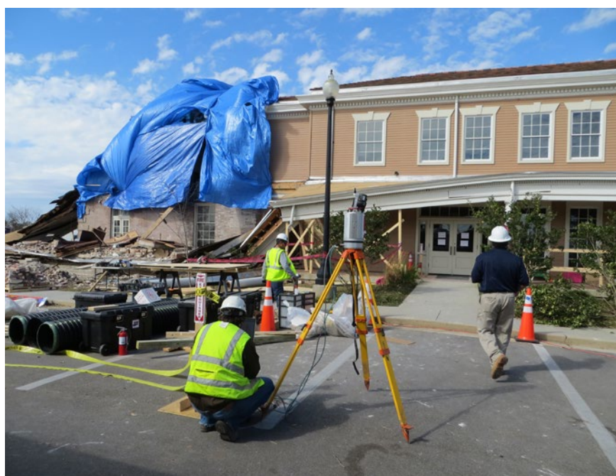
Right: EMC field crew scanning the Alumni House on the campus of the University of Southern Mississippi with a Riegl VZ400.
