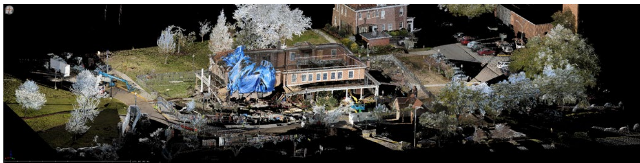
Colorized point cloud collected of the Alumni House on the campus of the University of Southern Mississippi with the Riegl VZ400.
