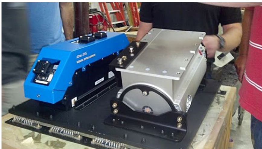
Figure 4 (a): Mounted with Riegl® VQ-480
