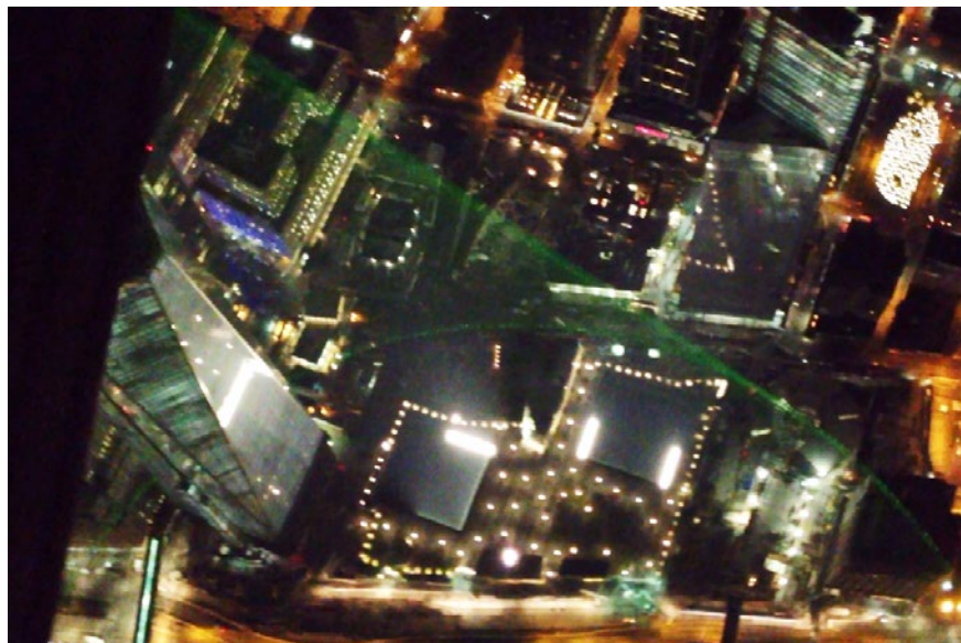
Figure 3: CZMIL laser cone and circular scan at the World Trade Center site. The blue-green laser is in the visible portion of the electromagnetic spectrum and is especially visible at night when there is no solar background.
