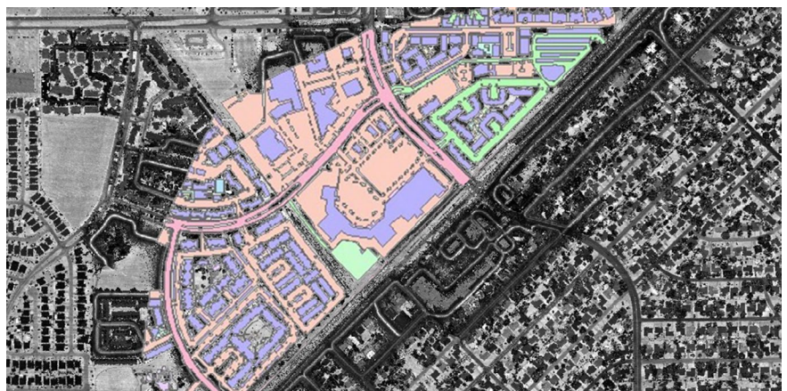
Figure 4: Fused LiDAR Point Cloud of a suburban jurisdiction with extracted and classified impervious features.
