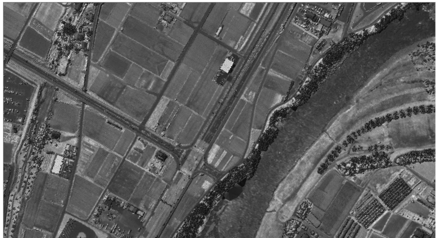
Figure 1: Intensity return from an Airborne Laser Scanner
