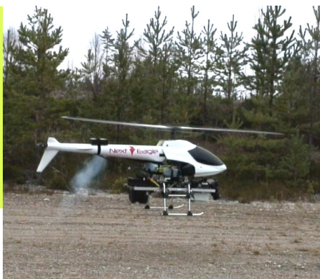
Unmanned aircraft JR GSR260Z equipped with laser scanner and high resolution camera used for the demonstration.
